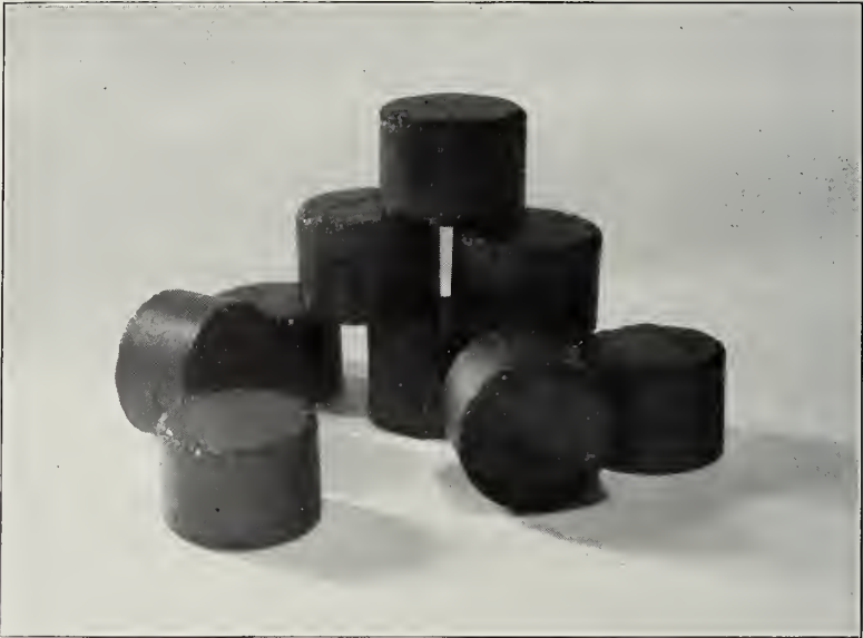
FIG. 12.—Cylindrical briquets formed by impaction, shown half size. The rounded edges are due to abrasion during tumbling tests.
